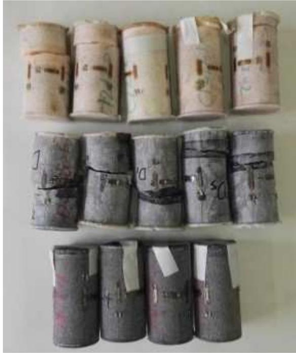
Fig. 2. Photographs of failed specimens after the direct tensile and uniaxial compressive tests. a – After direct tensile test, b – After uniaxial compressive test
